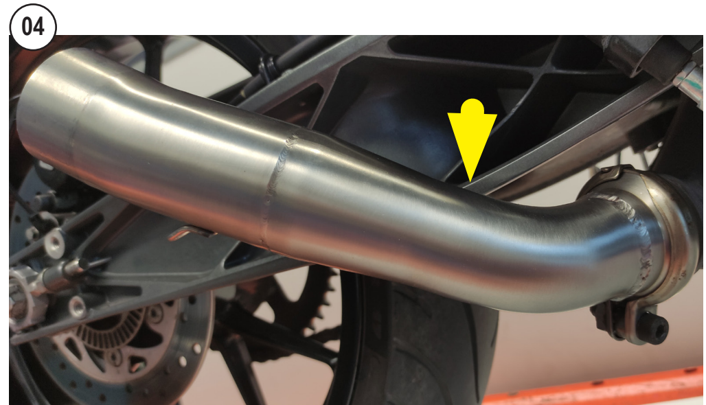
INSTALL THE PIPE - USE THE STOCK CLAMP
