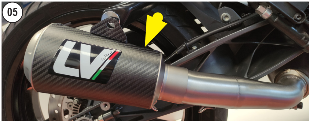
INSTALL THE MUFFLER
